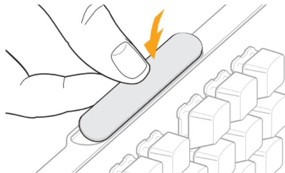
To install the signature plate, secure the top portion of the plate into the housing and then press the remainder of the plate in.
