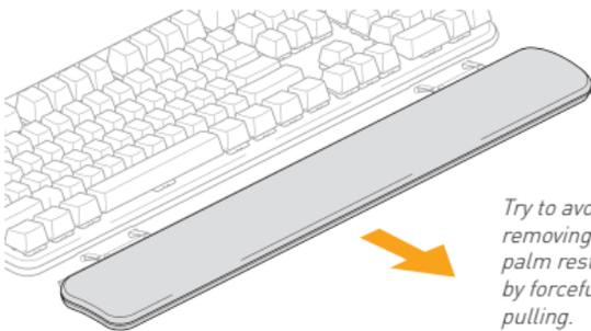
*Try to avoid removing the palm rest by forcefully pulling.*
