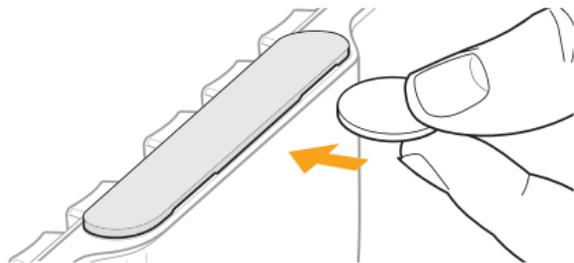
To remove the signature plate, simply pull the plate off from the bottom lip using a fingernail, coin or other thin apparatus.
